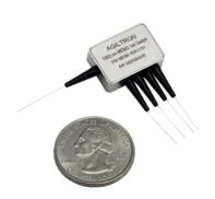
The MEMS 1x4 Latching Type Series Fiber Optic Switch connects optical channels by redirecting incoming optical signals into selected output fibers. This is achieved using a patent pending MEMS™ configuration and activated via an electrical control signal. It uniquely features rugged thermal activated micro-mirror movement instead of rotation.
